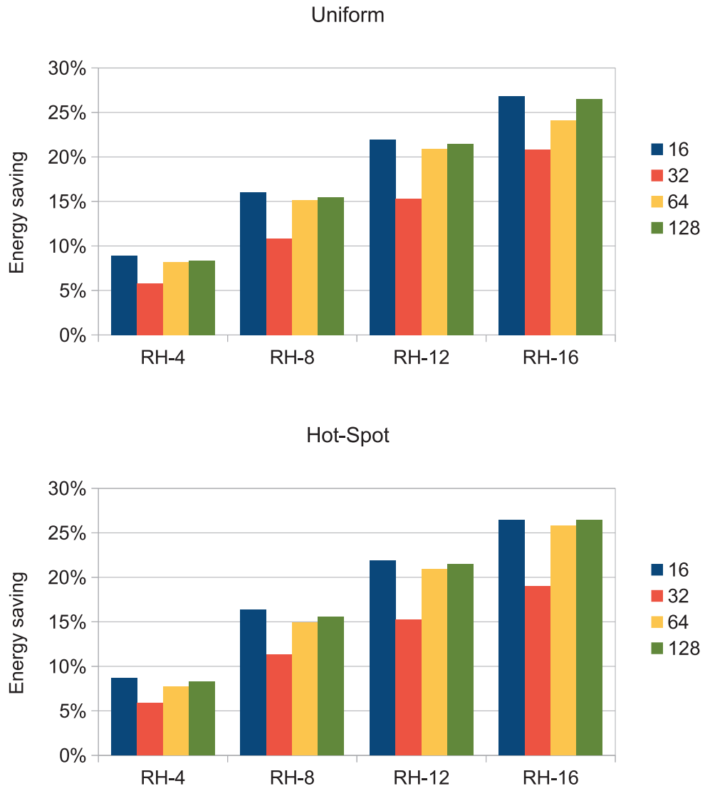
Figure 7.10: Energy saving for the for different flit size under uniform and hot-spot traffic scenarios.
