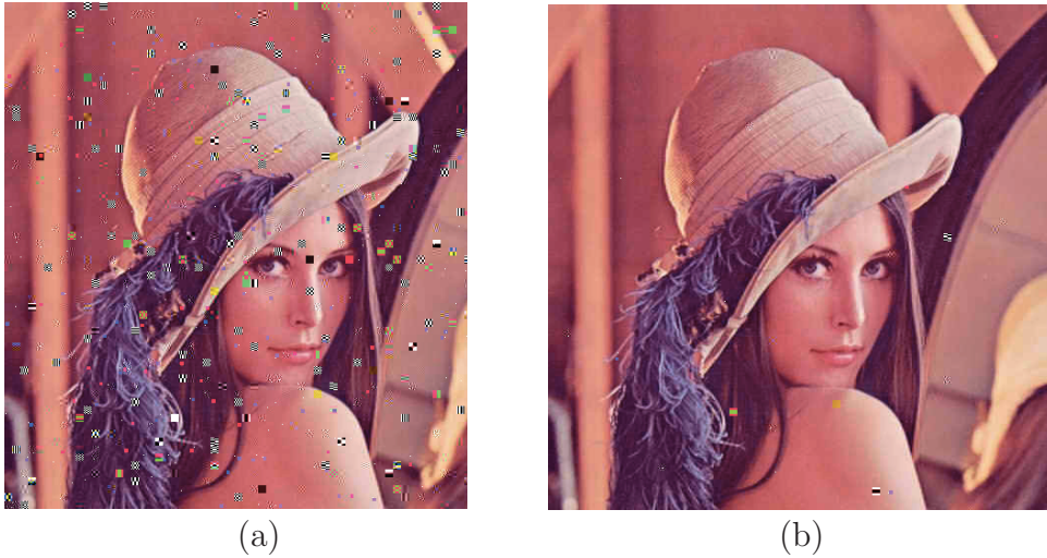
Figure 3.16: Image encoded and decoded based on the flow shown in Fig. 3.15 using two low voltage swing at 0.5 V (a) and 0.6 V (b).
