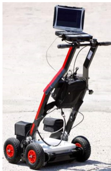
Figure 18 - Ground Coupled GPR IDS. University of Catania
