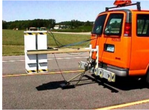
Figure 19 - Air coupled horn antenna. Source: http://www.ndt.net/article/ndtce03/papers/v110/fig2.jpg
