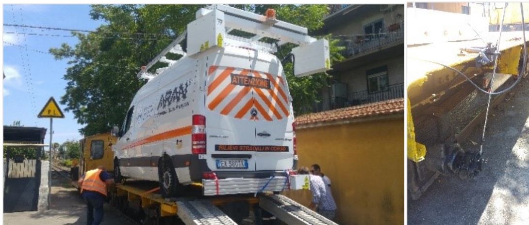
Figure 38 - LCMS configuration and DMI installed on the rail wagon wheel
