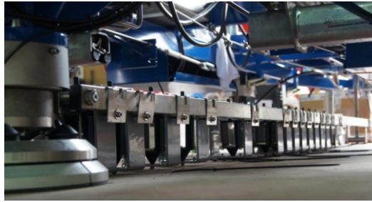
Figure 10 - Geophones bar. FWD Dynatest 8000 (University of Catania)
