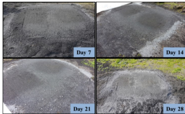
Figure 58 - Ashes cement stabilized at days 7-14-21-28
