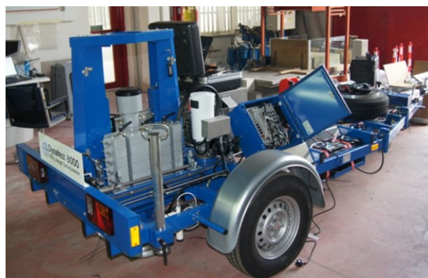
Figure 7 - Falling Weight Deflectometer 8000 (University of Catania)
