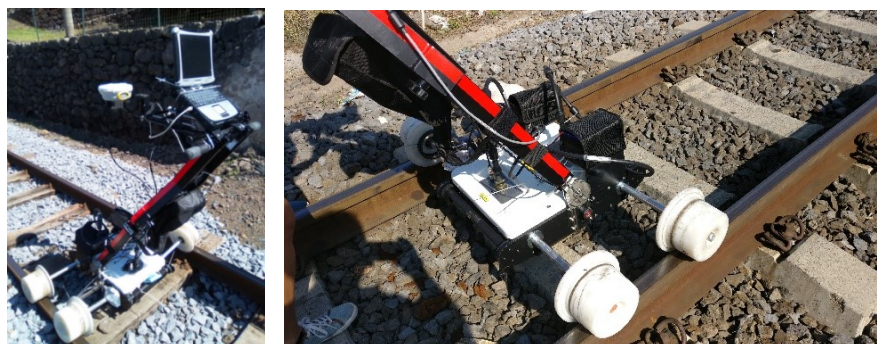
Figure 31- Ground Penetrating Radar adapted for rail inspection
