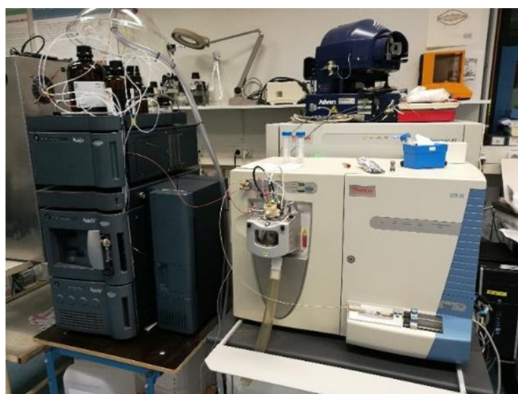
Fig. 20. Acquity Ultra Performance Liquid Chromatography system with a photodiode array (UPLC-PDA; Waters) coupled to LTQ Ion Trap-Orbitrap FTMS.
