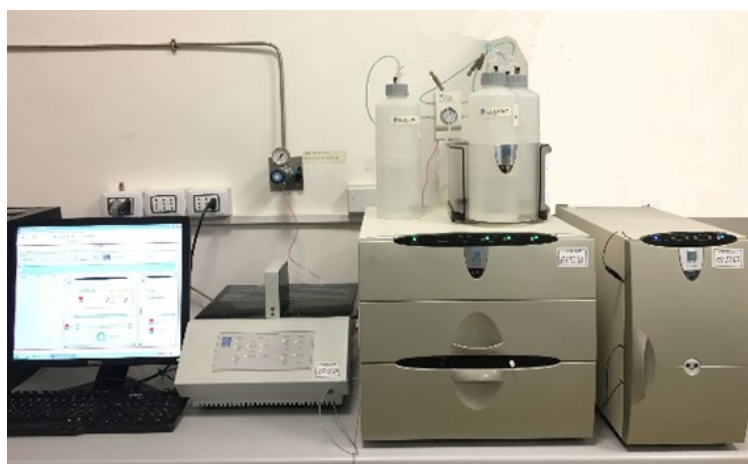
Fig. 17. Dionex ICS3000 (Thermo Scientific) Ion Chromatography System with Pulsed Amperometric Detection (line 1) and Conductometric Detection (line 2).
