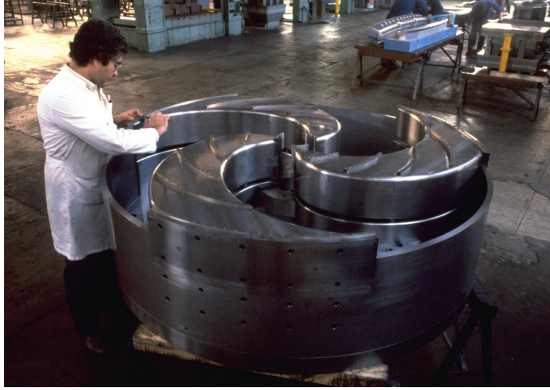
Figure 2.7: Pole sectors of the CS. Each hill is split in two parts. The upper part has rounded edge in order to facilitate the winding of the trim coils around it. The picture was taken in Milan before the installation of the CS in Catania.
