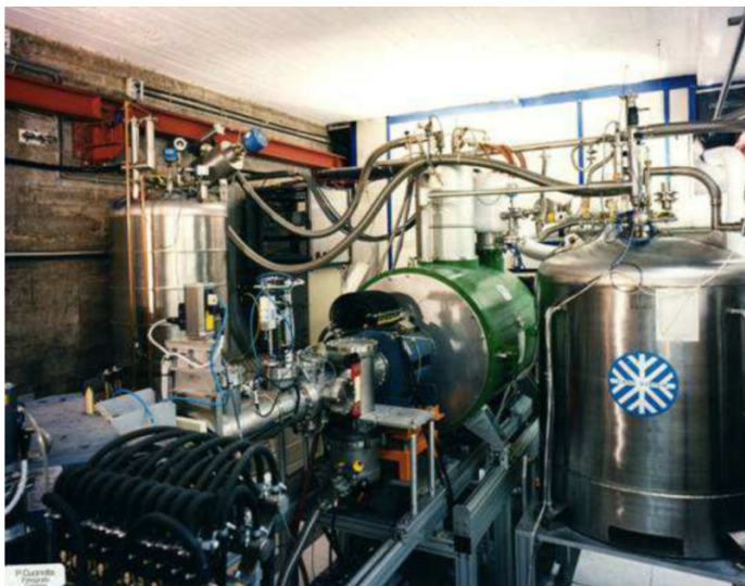
Figure 2.15: The SERSE ion source at INFN-LNS.
