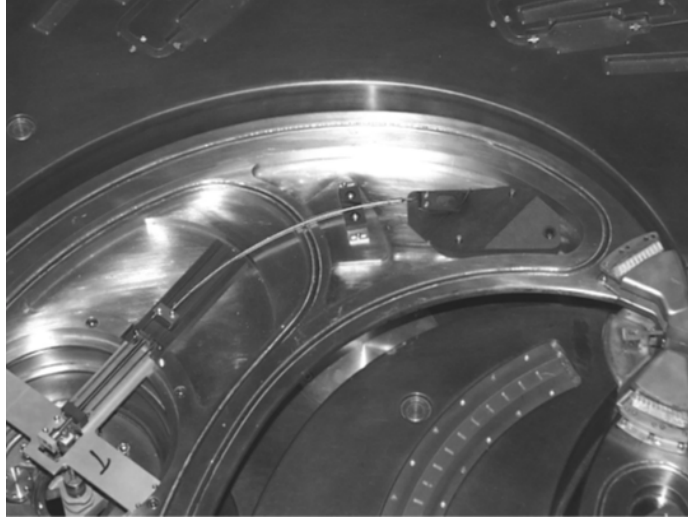
Figure 2.22: One of the three phase slits in the INFN-LNS Superconducting Cyclotron.
