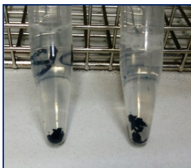
Fig. 4.7: Two examples of the solubility test performed on the paste obtained after 24h decantation, rinsing and removal of supernatant. In the picture, there are shown two Eppendorf test tubes containing the dark blue paste immersed respectively in 1M KOH (on the left) and in acetyl acetate (on the right).
