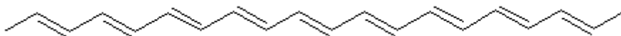
Fig. 1.1: Molecular structure of the polyacetylene, the simplest example of a conductive polymer with a conjugated structure.
