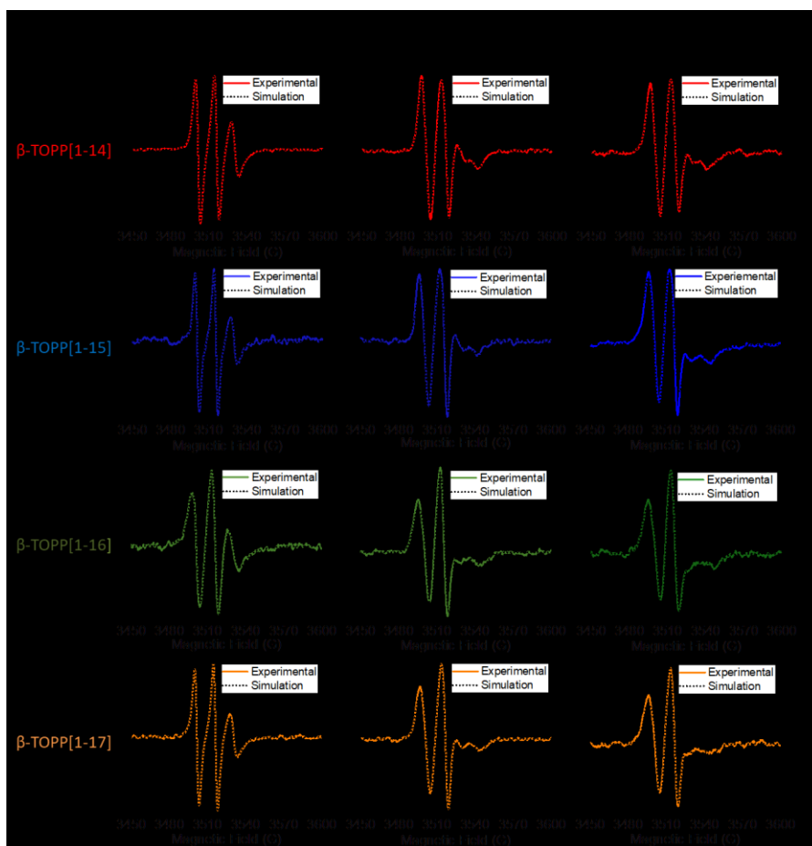
Figure 11.3 Normalized experimental (coloured solid line) and simulated (black dot line) CW-EPR spectra of \beta^3 -TOPP peptides in methanol solution with 20% glycerol (first column); MLVs of d_{31} POPC with Tris-HCl buffer in H_2O (second column); MLVs of POPC with Tris-HCl buffer in D_2O (third column).
