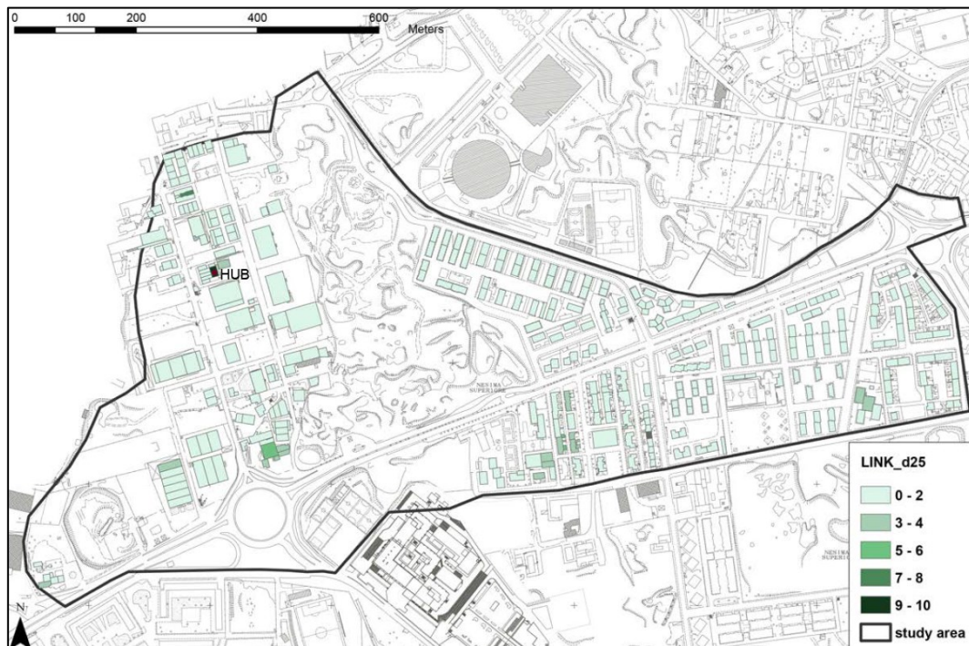
Fig.32 Map representing the node activated degree of nodes and the hubs for the configuration of scenario C_1 and at 25 m as maximum threshold distance d of connection
